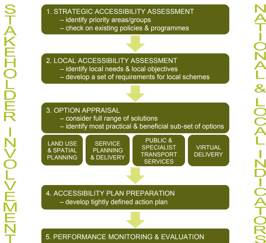
Figure 3.2: Recommended Process for Developing an Accessibility Strategy
